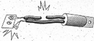
**Open-circuited collector temperature sensors keep the pump from turning on during the day. Open-circuited storage tank temperature sensors keep the pump running all night.**
