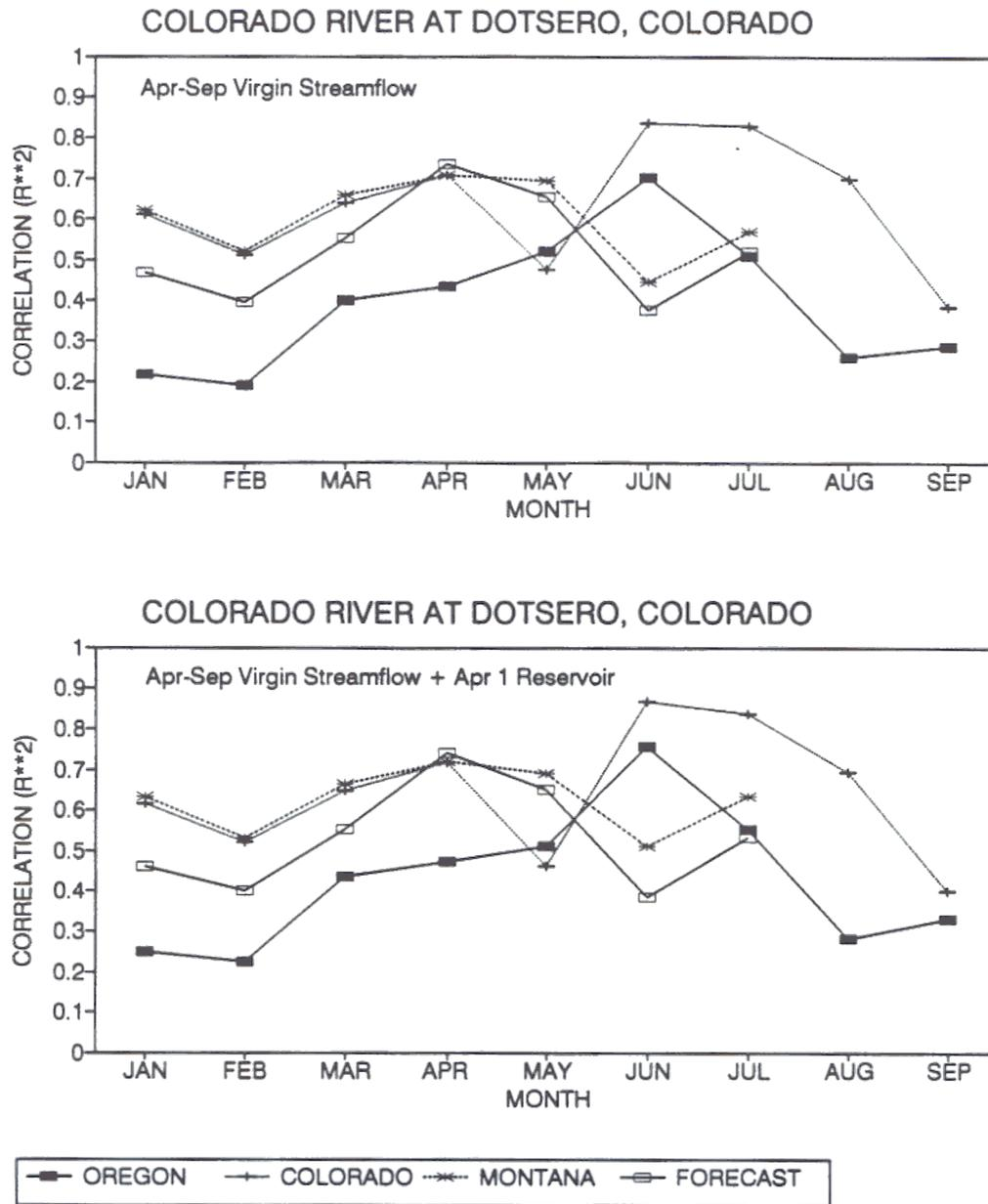
**Figure 9. Correlations of computed SWSI values with April-September virgin streamflow (top) and with April-September virgin streamflow plus active reservoir storage on April 1 for the Upper Colorado River above Dotsero, Colorado.**
