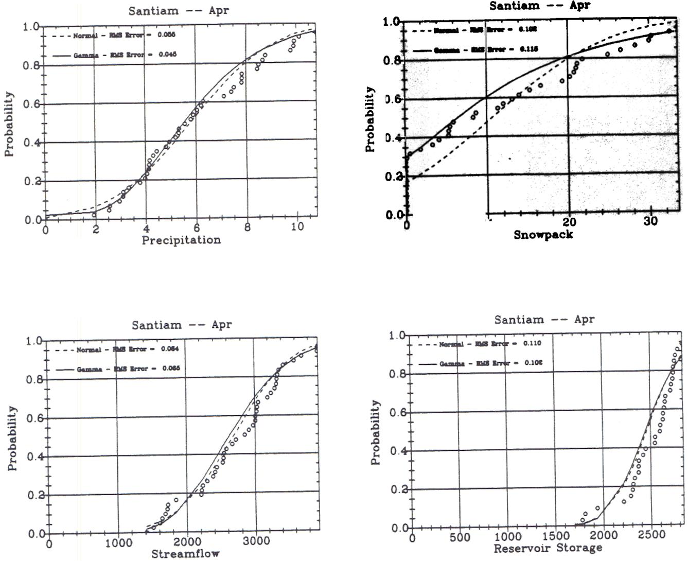
**Figure 4.** Observed distribution of monthly precipitation in the Santiam River Basin in Oregon for selected months and fitted distributions using a normal curve (dashed line) and a gamma curve (solid line). Root mean squared errors are shown in the upper left-hand corner to describe the goodness of fit.
