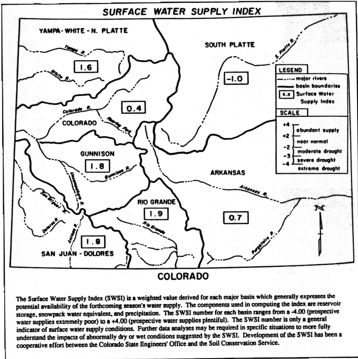
Figure 2. Example of a Surface Water Supply Index (SWSI) map.
