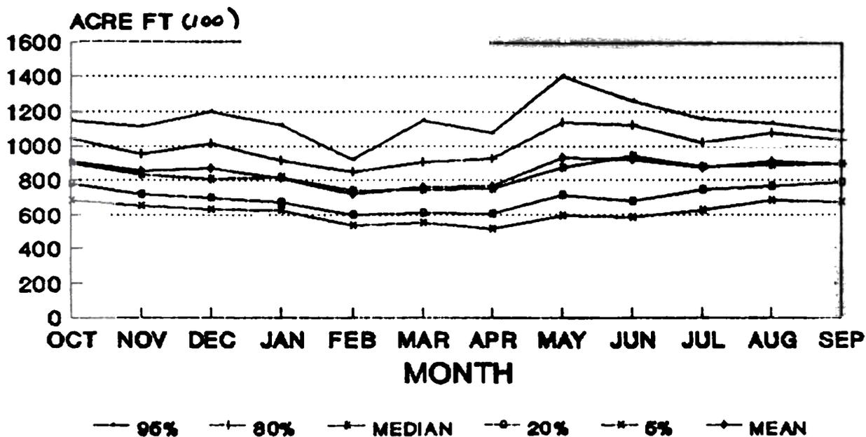
Figure 20. Nonexceedance probabilities, by month, associated with observed values of streamflow in the Deschutes River, Oregon.
