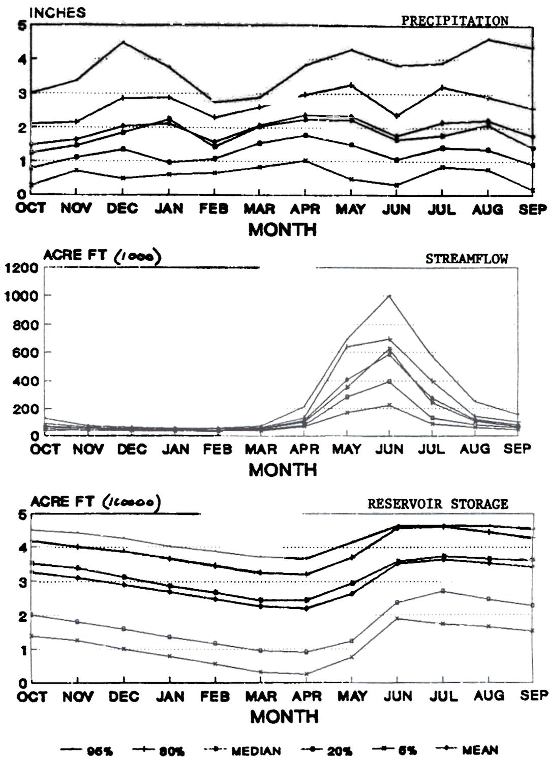
Figure 19. Nonexceedance probabilities, by month, associated with precipitation, streamflow and reservoir storage in the Colorado River above Dotsero, Colorado.
